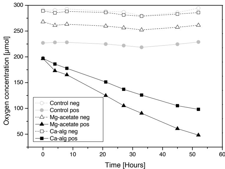
Figure 2. Shows dissolved oxygen measurements of the solutions in the bottles over time.
