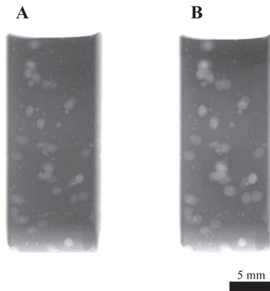
Figure 1. CT images taken of paste containing the capsules: (A) is an image taken after 4 min; and (B) taken after 180 min.
