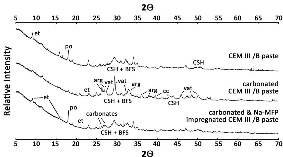
Figure 2: X-ray powder diffractograms of CEM III /B cement pastes; Na-MFP treatment after carbonation causes the formation of secondary cement phases.
