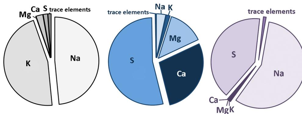
Figure 1: Main element concentrations of slag-rich cement paste pore solutions in percent; left: untreated CEM III /B; middle: carbonated CEM III /B; right: carbonated and subsequently Na-MFP impregnated CEM III /B.
