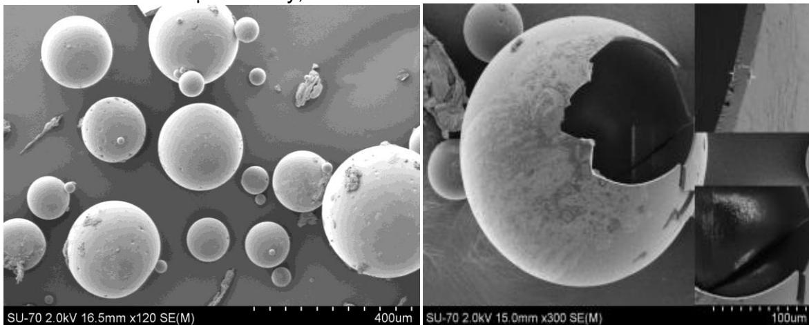
Fig. 1 SEM image of PF/DCPD microcapsule showing: (a) morphology, (b) fractured shell
