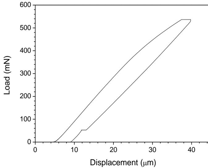
Fig. 2 the load–displacement curve of PF shell on continuous stiffness model
