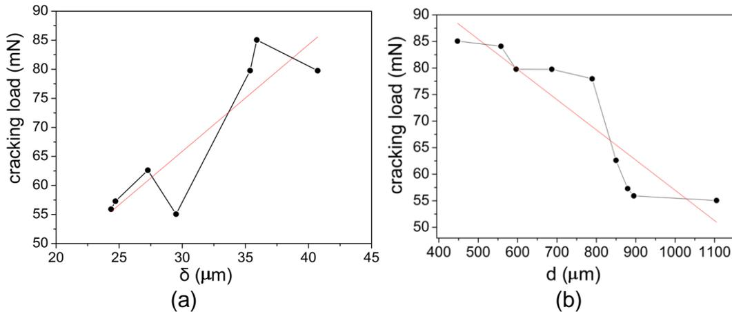
Fig. 3 Cracking load varies with (a) microcapsule’s diameter  $d$ , (b) shell’s thickness  $\delta$
