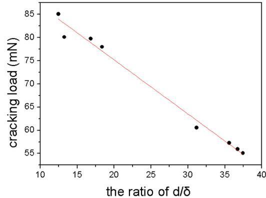
Fig. 4 The strict linear relationship between cracking load and  $d/\delta$
