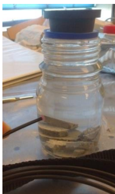
Figure 1: Non-invasive oxygen measurement for oxygen consumption in time. M = control mortar, M+HA+S = mortar with healing agent and bacterial spores.
