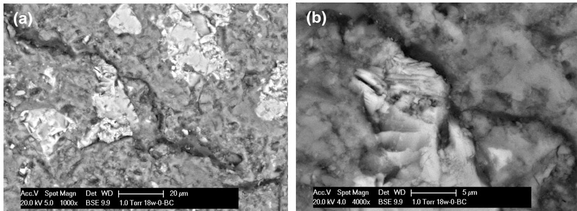
Figure 2: Mineral formation on the crack surface of a bacteria-based specimen. (a) ESEM image 1000xmagnification. (b) ESEM image 4000xmagnification.
