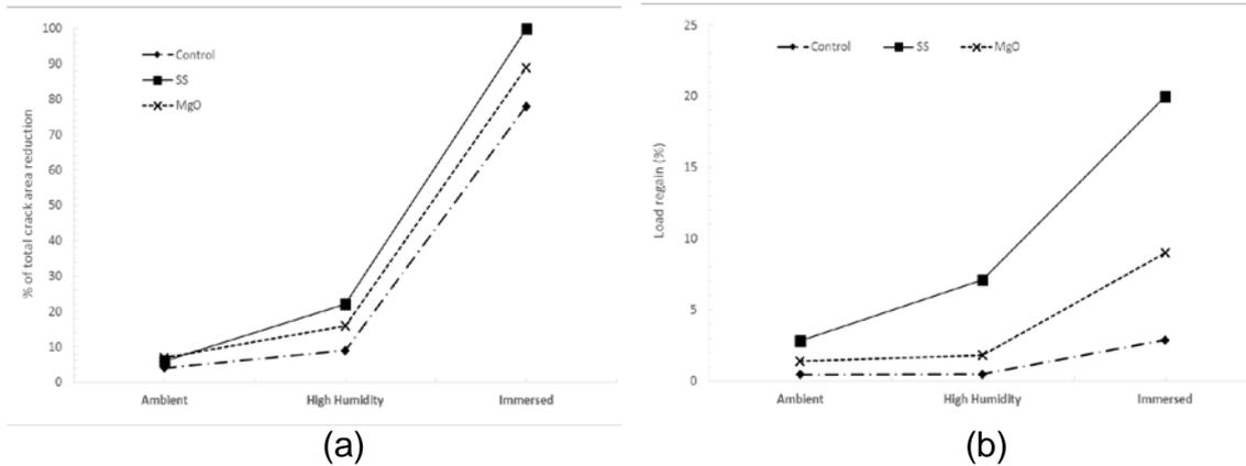
**Fig. 1.** (a) % reduction of the total crack closure area for all exposure conditions and (b) % regain of load for all exposure conditions
