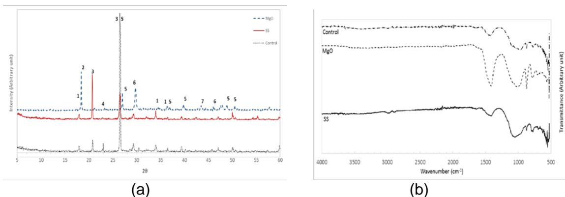
**Fig. 3.** (a) XRD patterns for all healing products (1:  $\text{Ca}(\text{OH})_2$ ; 2:  $\text{Mg}(\text{OH})_2$ ; 3:  $\text{SiO}_2$ ; 4: Ettringite; 5:  $\text{C}_3\text{S}/\text{C}_2\text{S}$ ; 6:  $\text{CaCO}_3$ ; 7:  $\text{MgO}/\text{MgCO}_3$ ) and (b) FTIR spectra of the healing products developed in specimens stored under water.
