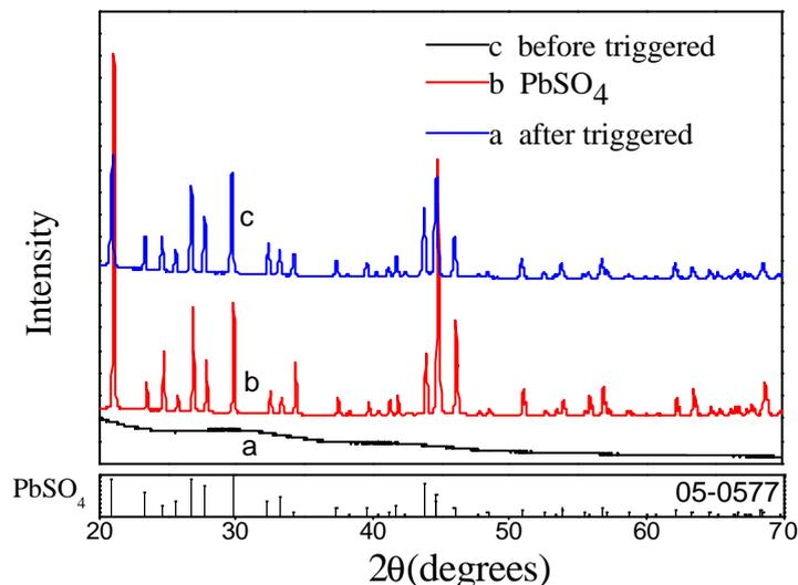
Fig.5 XRD of  $\text{PbSO}_4$  powders and the shell  $\text{PbSO}_4$  embedded in before and after  $\text{Cl}^-$ -triggered
