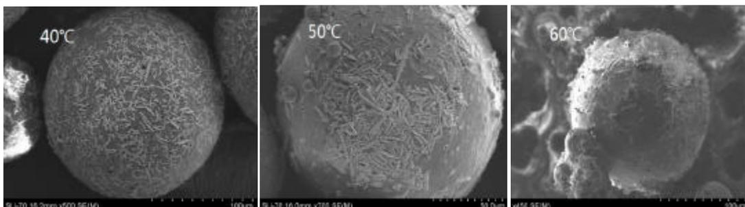
Fig.2 SEM images of microcapsules formed at different temperatures
