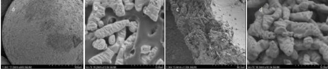
Fig. 3 SEM images of: (a) microcapsule, (b) impaction of  $\text{PbSO}_4$ , (c) cross-section of shell, (d)  $\text{PbSO}_4$  powders.
