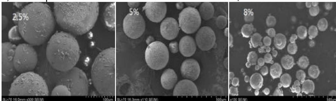
Fig.1 SEM images of as-prepared microcapsules with different concentration of PVA
