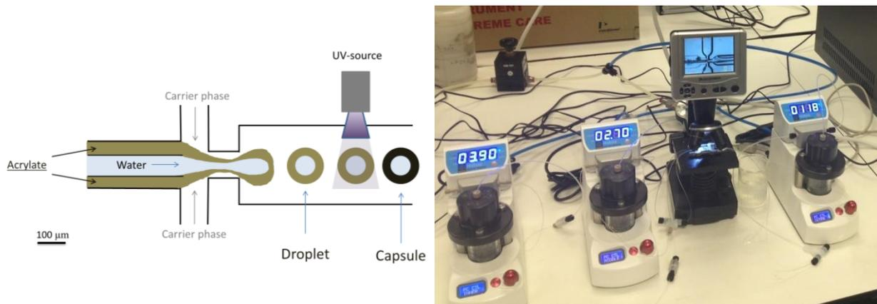
Figure 1 - Schematic representation of the production of microcapsules using microfluidics (left) and set-up of the experiments (right).
