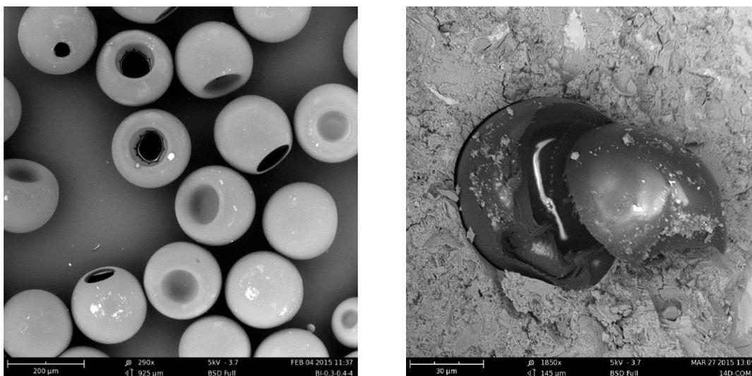
Figure 3 – SEM images of the microcapsules (*left*) and the casted broken capsule (*right*).
