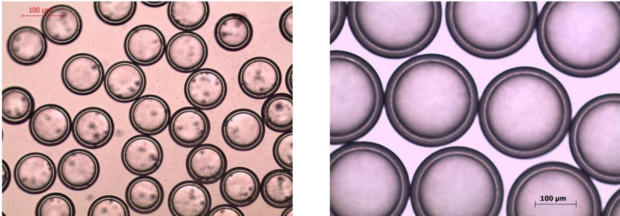
Figure 2 – OM images of double emulsion produced at the flow rate of 0.7-0.35-80  $\mu\text{L}/\text{min}$  (left) and 5-6.7-67  $\mu\text{L}/\text{min}$  (right), for the inner, middle and outer fluid, respectively.
