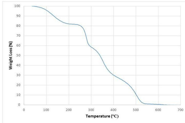
Figure 4 - TGA analysis of the microcapsules.
