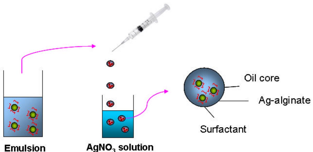
Fig.1 Schematic of Ag-alginate capsules encapsulated oil cores.
