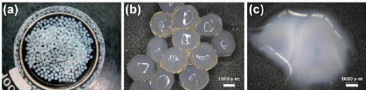
Fig. 2 (a) Ag-alg capsules, (b) Optical image of Ag-alg capsules, (c) disintegrated Ag-alginate capsule when exposed to chloride ions
