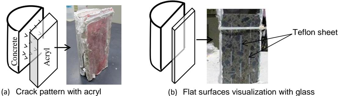
Figure 3: Specimens for direct visual observation of water flow
