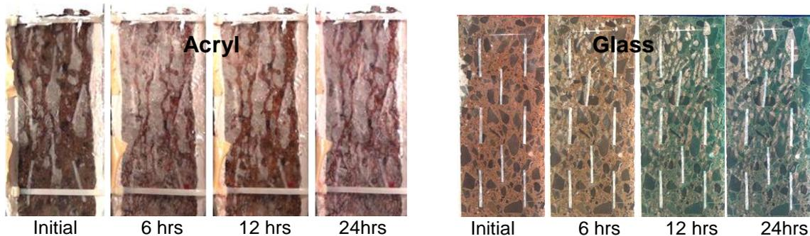
Figure 4: Air bubbles observed through acrylic resin and glass interfaces
