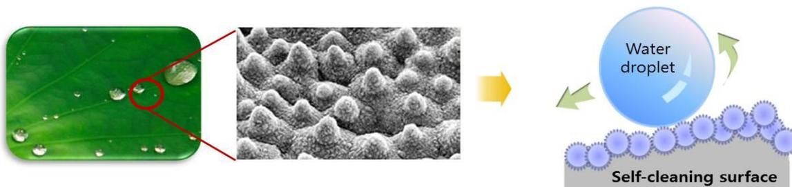
Figure 1: Schematic of self-cleaning surface mimicking lotus leaf
