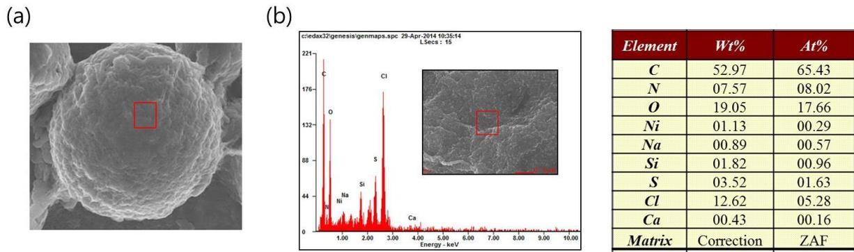
Figure 3 : Evaluation of surface nano structure by PANI(polyaniline) polymerization by FE-SEM and EDAX
