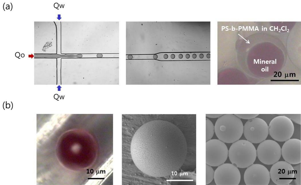
Figure 2 : Visualization of encapsulating mineral oil in the microchannel
