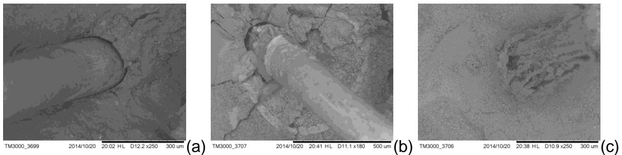
Figure 3 : detail of fibre-matrix interface in : (a) non healed steel HPFRCC; (b) healed steel HPFRCC and (c) healed sisal+steel HPFRCC.
