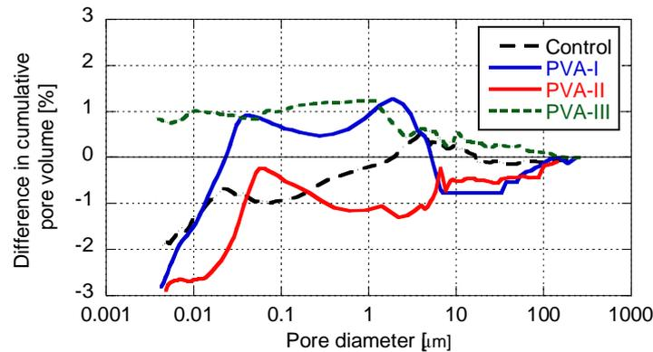
Figure 4: Difference of cumulative pore volume between before and after curing.
