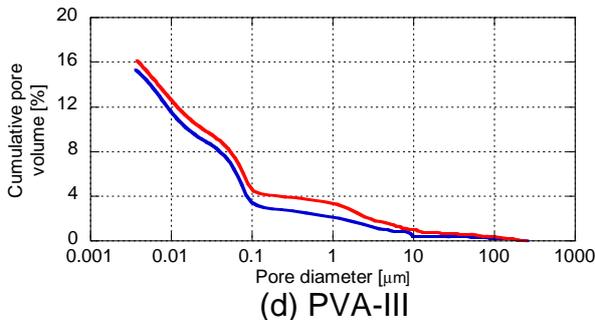
Figure 3: Pore size distribution before curing (just after 300 freeze/thaw cycles) and after 28 days of curing
